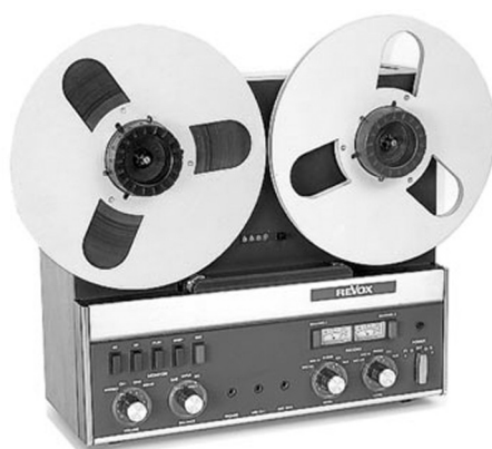
Figure 2. ReVox A77 reel-to-reel tape recorder.
